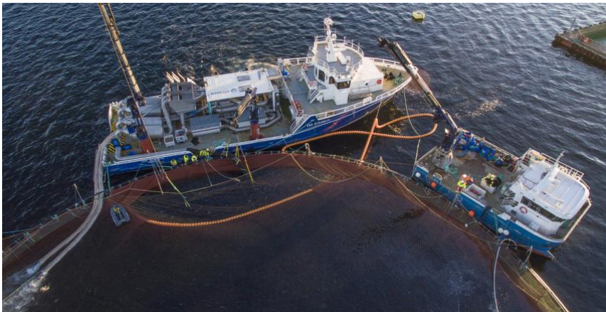
Figure 2.4: A vessel with an onboard Thermolicer system performing a delousing operation, supporting service vessel is seen to the right. (TU.no (2018))
