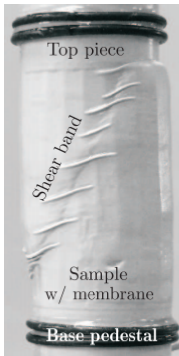
Figure 2.5: Observable shear band in a modified triaxial cell[12]
