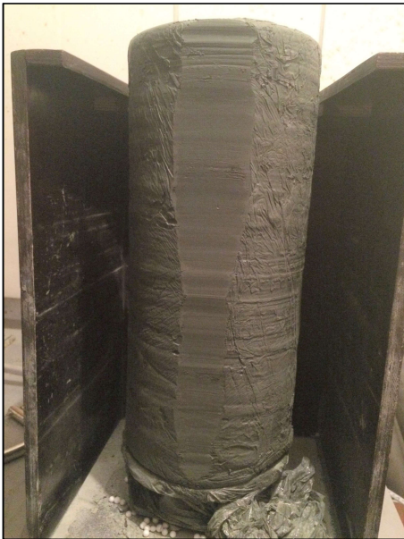
Figure C.1: Mini-block showing dark, silt layers
