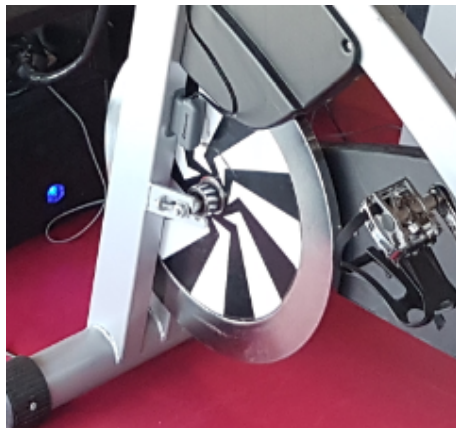
Figure 7.2: Bicycle wheel with sensor.
