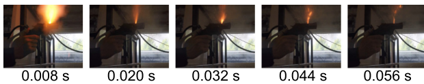
Figure 9. Recorded signal at hydrophone H2 in air (black) and H1 in water (blue) according to Fig. 6. The source was fired at z_s = -0.3 m. The signal is filtered with a 10–100 Hz (top), 10–200 Hz (middle) and 10–300 Hz (bottom) bandpass filter. Photos show a side view of the signalgun while it is fired according to different times.
