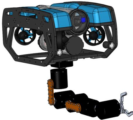
Fig. 5: A 3D model of the BlueROV2 ROV and SeaArm manipulator arm within the Solidwork 3D modelling environment.
