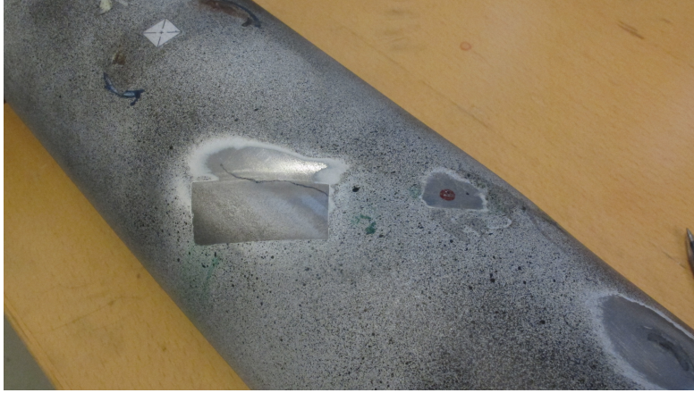
Figure 4.8: Shows location of crack in 45 deg. dent. Pipe was exposed to a cyclic pressure of 4-40[Bar] with fatigue life of 69k cycles.
