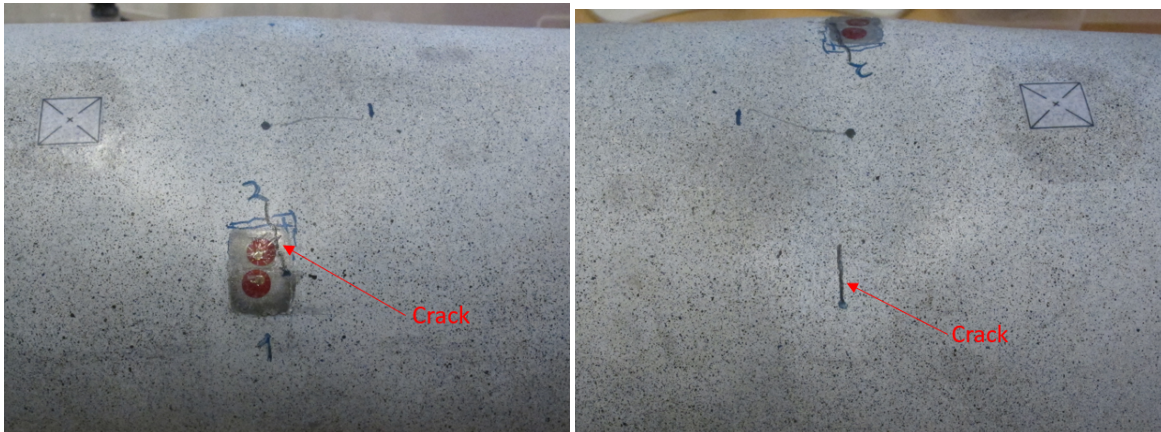
Figure 4.4: Shows location of two cracks on the same pipe in 90 deg dent. Pipe was exposed to a cyclic pressure of 5-50 [Bar] with fatigue life of 68k cycles.
