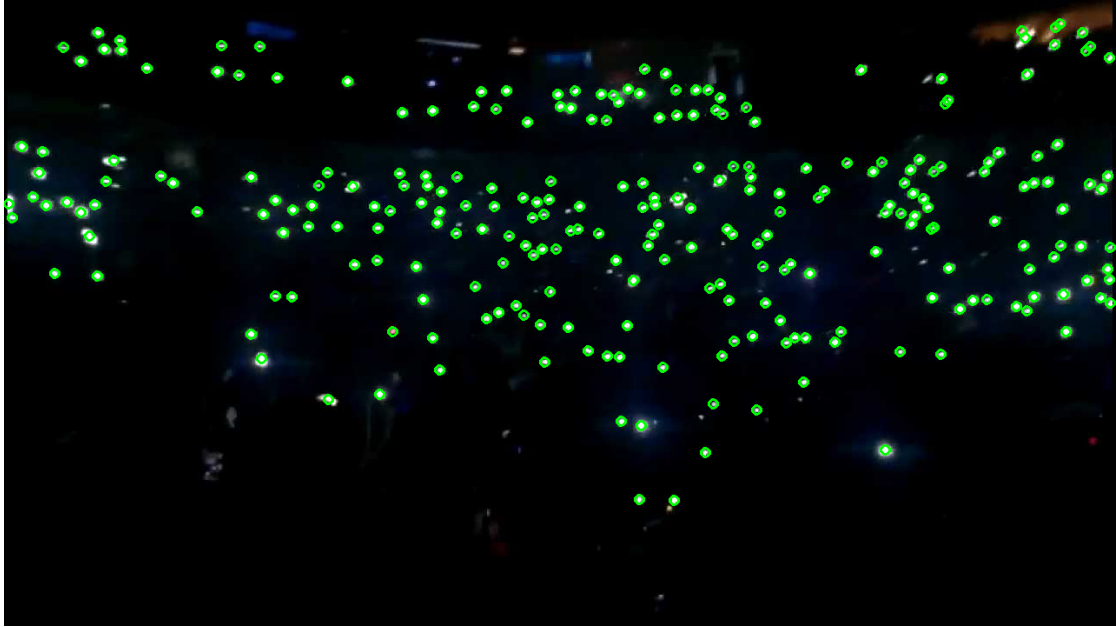
Figure 4.8.: Example of manual binary thresholding, using a value of 240, applied to a real-world image sample with 257 devices.
