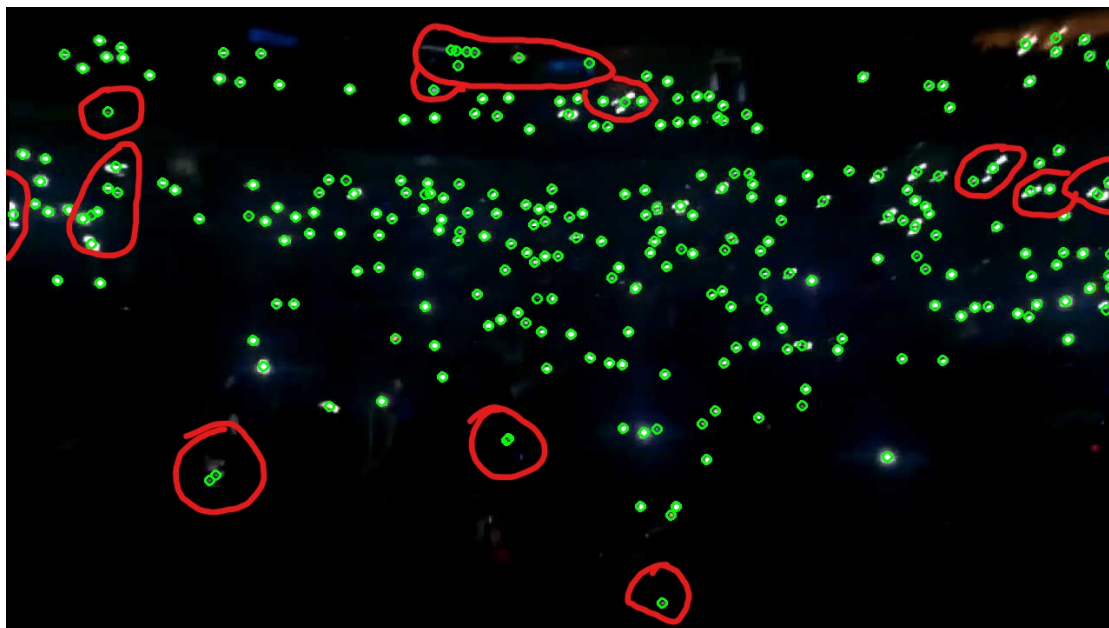
Figure 4.7.: Example of Otsu’s Method thresholding applied to a real-world image sample with 257 devices. Green circles indicate devices that were detected by the algorithm. Red circles highlight incorrect detections.
