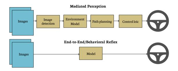
Figure 2.5: The difference between end-to-end and mediated perception to autonomous driving with camera input.
