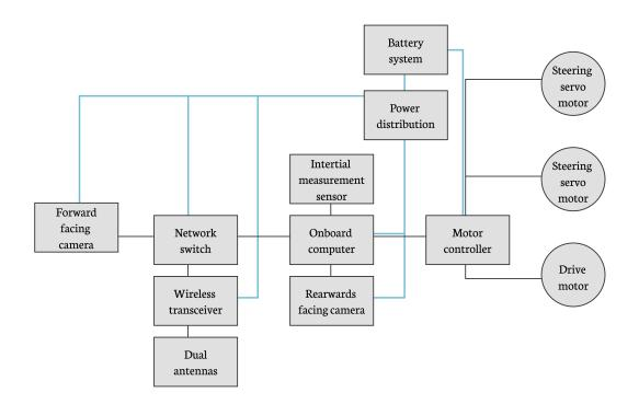
Figure 2.11: A block diagram of the hardware components in the SPURV car and how they are connected. The blue lines denote power distribution.
