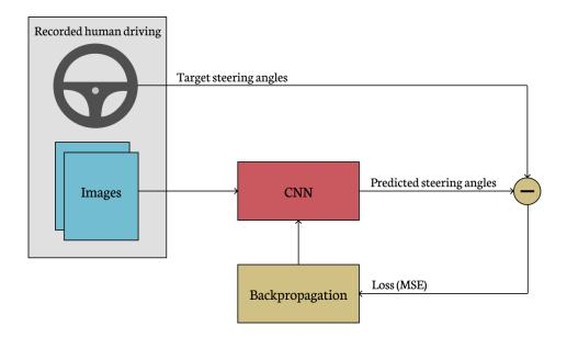
Figure 2.6: An overview of the PilotNet system.
