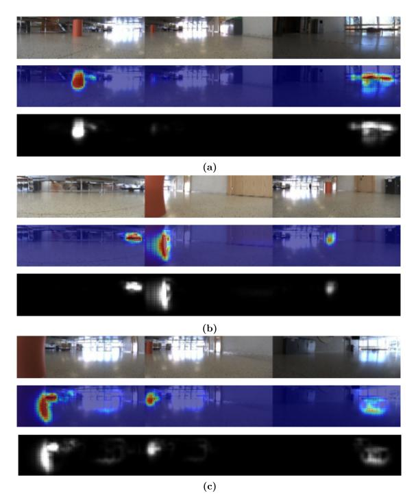
**Figure 4.17:** VBP heat maps for *SpatialSpurvPilotExtended* trained on the marker turning task. The leftmost images are the most recent in the spatial history, and the following images are 80 frames apart, as explained in Figure 3.22.
