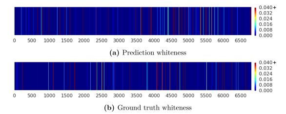
**Figure 4.13:** A visualisation of the whiteness of the predicted steering angle by SpatialSpurvPilot for each image in the validation set (a), compared to the ground truth whiteness (b). The whiteness is measured in rad<sup>2</sup>/frame.
