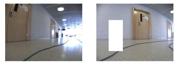
Figure 3.10: To the left an example of an image that suffers from occlusion from light reflection. To the right is an example of an image augmented by erasing a random square.
