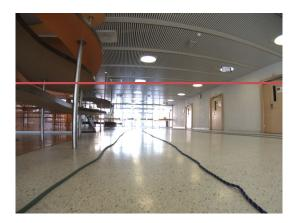
Figure 3.6: Everything above the red line, the top 35%, was considered irrelevant and removed from the images.
