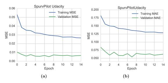
Figure 4.8: Training history plots showing the development in MSE and MAE during training of the  $SpurvPilot_{Udacity}$  model.
