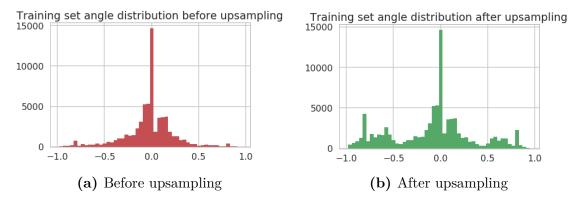
Figure 3.17: Histograms showing the distribution of angles of the ground truth in the validation set for the SPURV lane following task before and after the upsampling of angles larger than 0.5 radians by a factor of 5.
