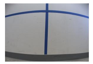
**Figure 3.13:** An example of the fish eye-like distortion in the forward camera on the SPURV. In reality, all lines in this scene are straight.
