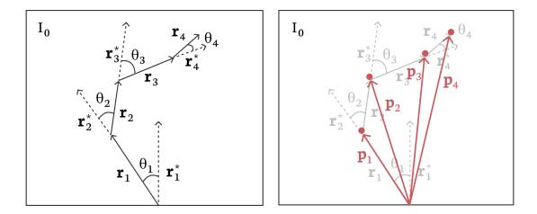
Figure 3.12: Left: An illustration of  $I_0$  with future car paths represented as vectors  $\mathbf{r}_i$ . Right: An illustration of how the sum  $\mathbf{p}_i$  of each vector  $\mathbf{r}_i$  directly maps to the coordinates of points in the path visualisation.
