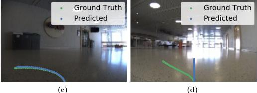
Figure 4.15: Visualisations of predicted driving paths by *SpatialSpurvPilot*, compared to ground truth paths, on a selection of images from the validation set for the marker turning task.
