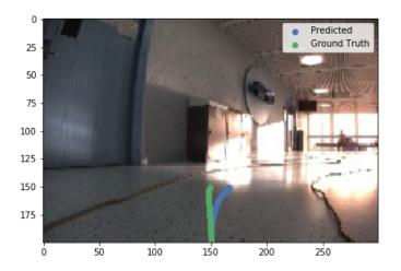
Figure 3.14: Arbitrary output from the path visualisation implementation. The two paths illustrate the approximate path of the car two seconds ahead in time, for both the ground truth and the predictions.
