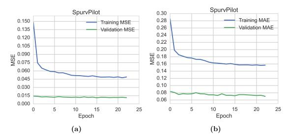
**Figure 4.1:** Training history plots showing the development in MSE and MAE during training for the SPURV lane following task.
