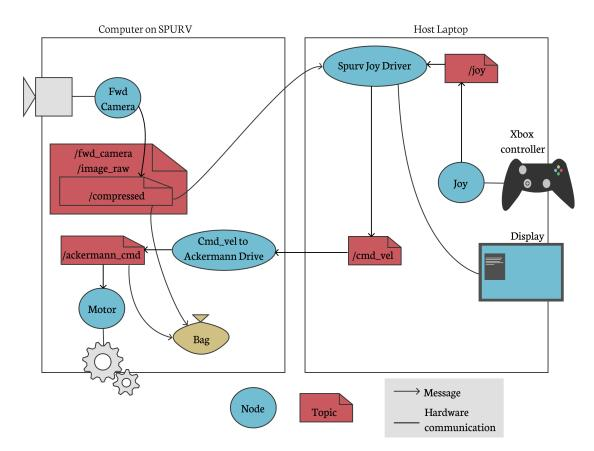
Figure 3.2: The ROS computation graph during data collection using the SPURV. The Xbox controller is used to steer the SPURV, while the display shows the images from the forward camera. Steering commands and images are saved in a ROS bag. Note that the details between /ackermann\_cmd and the actuators are omitted.
