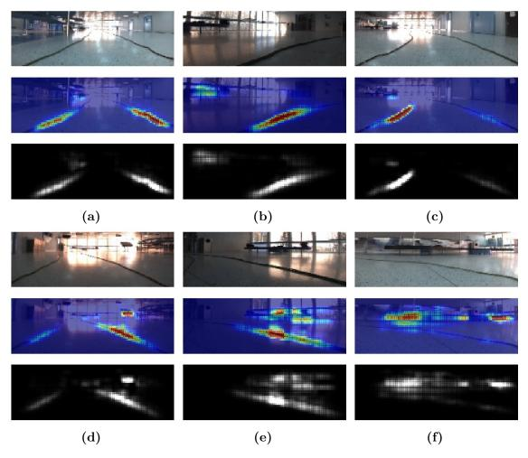
**Figure 4.4:** The *SpurvPilot*'s VBP heat maps on a selection of images from the test set. The bottom row shows examples where the model focuses on undesired features in the image.
