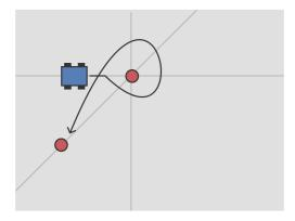
**Figure 3.23:** The maximal turn of  $2\pi + \frac{\pi}{4} = \frac{9\pi}{4}$  radians the SPURV would have to make.
