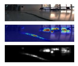
Figure 3.15: An arbitrary output of the VBP implementation. The visualisation shows that the network focuses on wanted features in the lane, but also reveals undesired focus on the benches in the back of the image.
