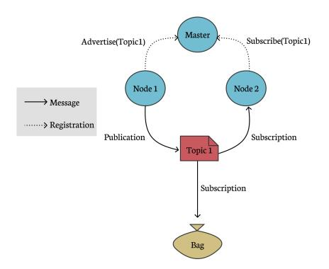
Figure 2.12: A simple figure of the relevant graph concepts of ROS and how they are connected through message passing. Node 1 first notifies the master that it wants to advertise to topic 1. Node 2 registers its subscription to topic 1. Any messages published to topic 1 will then be passed on to node 2. If a bag is recording topic 1, it will also receive these messages.
