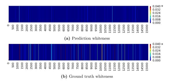
Figure 4.2: A visualisation of the stability of the predictions, i.e. the whiteness of the predicted steering angle for each image in the test set (a), compared to the ground truth whiteness (b). The whiteness is measured in  $rad^2/frame$ .
