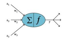
Figure 2.1: A single node in a neural network.
