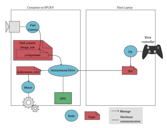
Figure 3.5: The ROS computation graph during autonomous driving using the SPURV. The Xbox controller is used only for turning on and off autonomous mode, and does not output steering commands. Note that the details between /ackermann\_cmd and the actuators are omitted.
