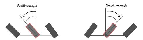
Figure 3.4: An illustration of what the Ackermann steering angles in ROS represent. The imaginary wheel with the red border represents the Ackermann steering value. The red wheel is rotated with the average angle of the front left and right wheel. When the car is turning left, the steering angle is positive, and its value is negative if the car is turning right.
