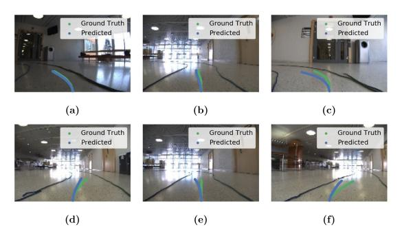
Figure 4.3: Visualisations of predicted driving paths, compared to ground truth paths, on a selection of images from the test set.
