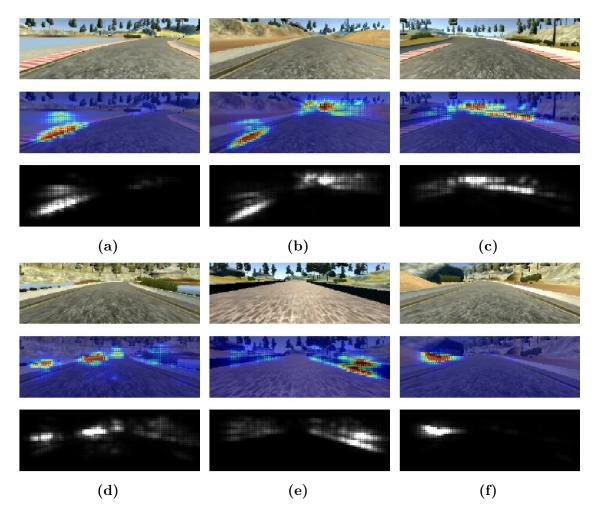
**Figure 4.10:** VBP heat maps of a selection of images from the validation set on the  $SpurvPilot_{Udacity}$  model.
