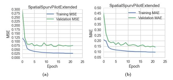
**Figure 4.12:** Training history plots showing the development in MSE and MAE during training of *SpatialSpurvPilotExtended* for the marker turning task.
