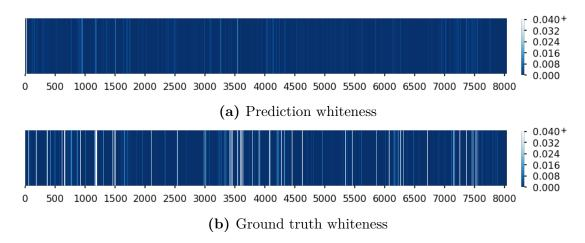
Figure 4.9: A visualisation of the whiteness of the predicted steering angle for each image in the Udacity Simulator test set (a), compared to the ground truth whiteness (b). The whiteness is measured in  $rad^2/frame$ .
