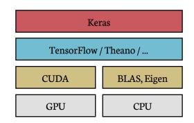
Figure 2.13: The deep learning software and hardware stack with TensorFlow and Keras.
