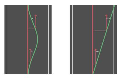
**Figure 2.9:** Examples of two model-predicted driving paths (green lines), compared to straight forward target path (red lines). The left driving path is acceptable, while the right path is erroneous. However, both paths will have approximately the same error compared to the straight forward path, as only the angles are compared.
