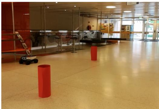
(e) External camera screenshot of the SPURV driving straight although there are markers around
