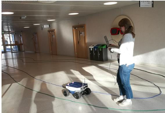
**Figure 3.3:** An image taken during the data collection process in the lane following task. One person walks behind the SPURV carrying the host laptop while simultaneously steering with an Xbox controller.
