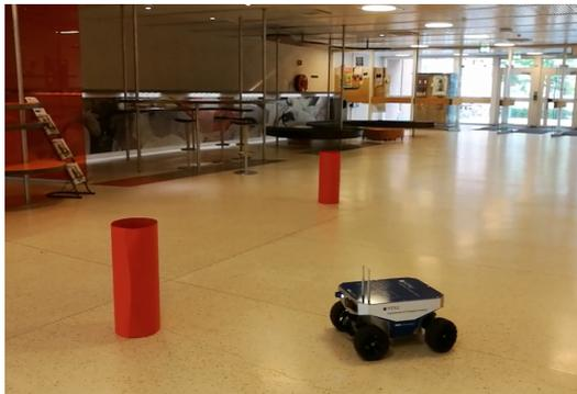
(c) External camera screenshot as SPURV drives straight when it is not supposed to
