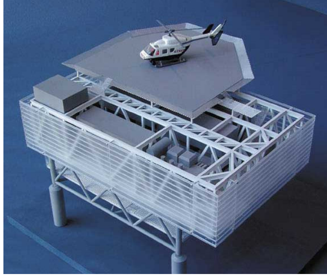
Figure 4.2: The Horns Rev offshore transformer
