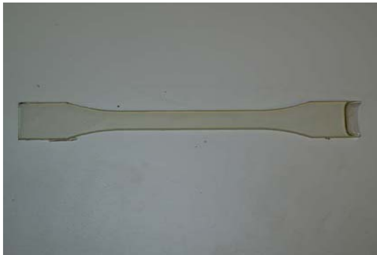
Fig. 10: Dog bone shaped epoxy sample (4 mm X 115 mm X 10 mm) used for mechanical (stress-strain) measurements.
