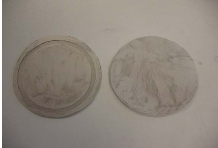
Fig. 9: Epoxy disc sample (1mm thick X 94 mm diameter ) used for dielectric characterization.
