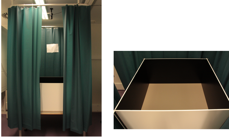
Figure 3.3: The apparatus set-up for cognitive tests, showing the recording camera, distal cue, curtains and the apparatus itself.
