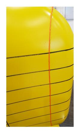
Figure 3.4: Tripwire on a model ship bulb.
