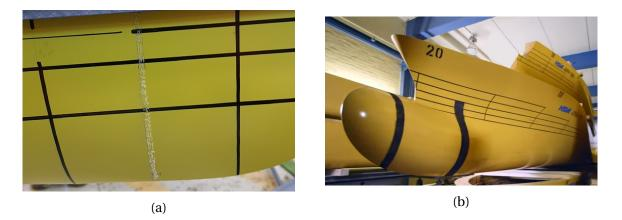
Figure 3.6: Sand strips as turbulence stimulation for two ship models.
