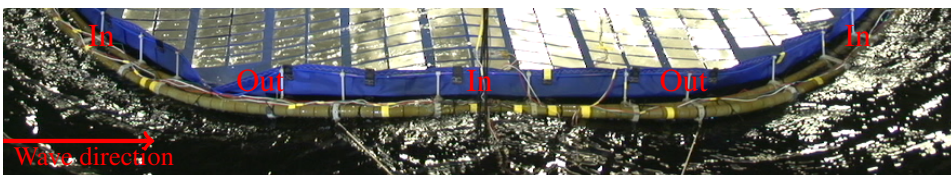
Figure 3.21: Motion in short period waves. Run 3220, H = 1.67\text{m} , T = 4.00\text{s} and steepness = 1/15 .
