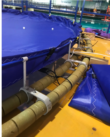
Figure 2.1: Close-up showing how the membrane is fastened to the floating collar, as well as the brackets and the railing.
