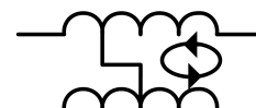
Figure 3.7: Phase-phase short. Depending on the inductance and resistance of the short circuited path, and the flux linking it, a large circulating current can occur.
