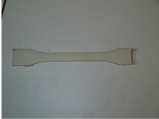
Figure 2: “Dog bone” shaped Epoxy sample
