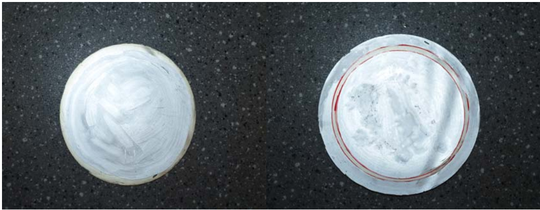
Figure 5: Epoxy samples casted in machine. With silver painted electrodes.
