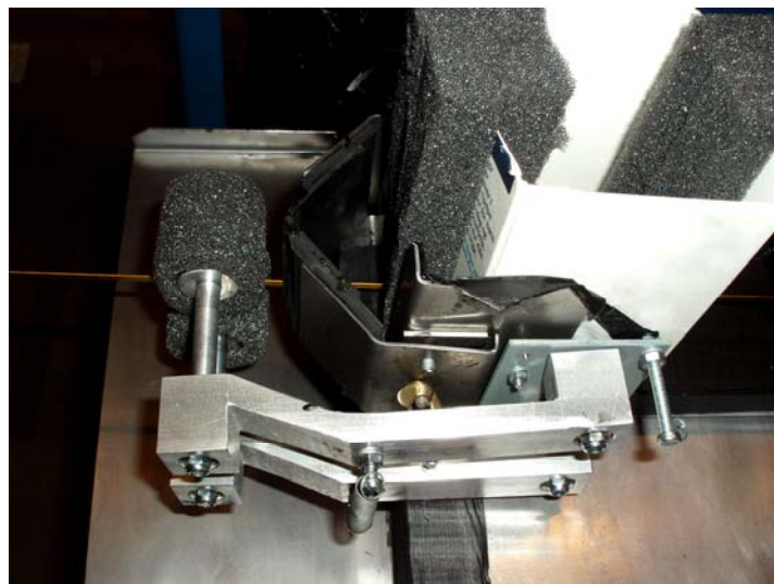
Figure 2-6: The epoxy feeder with the wiper and roller mechanism.
