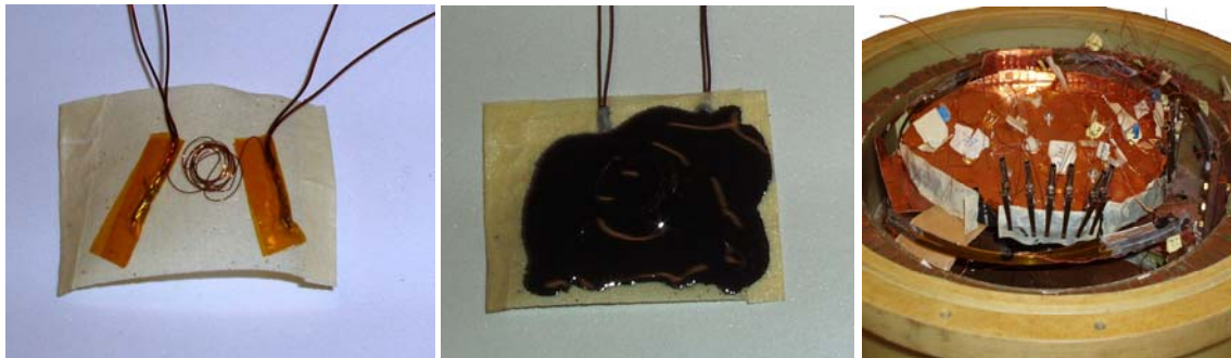
Figure 4-9: Simple way of attaching wires to the samples by using paper tape.
