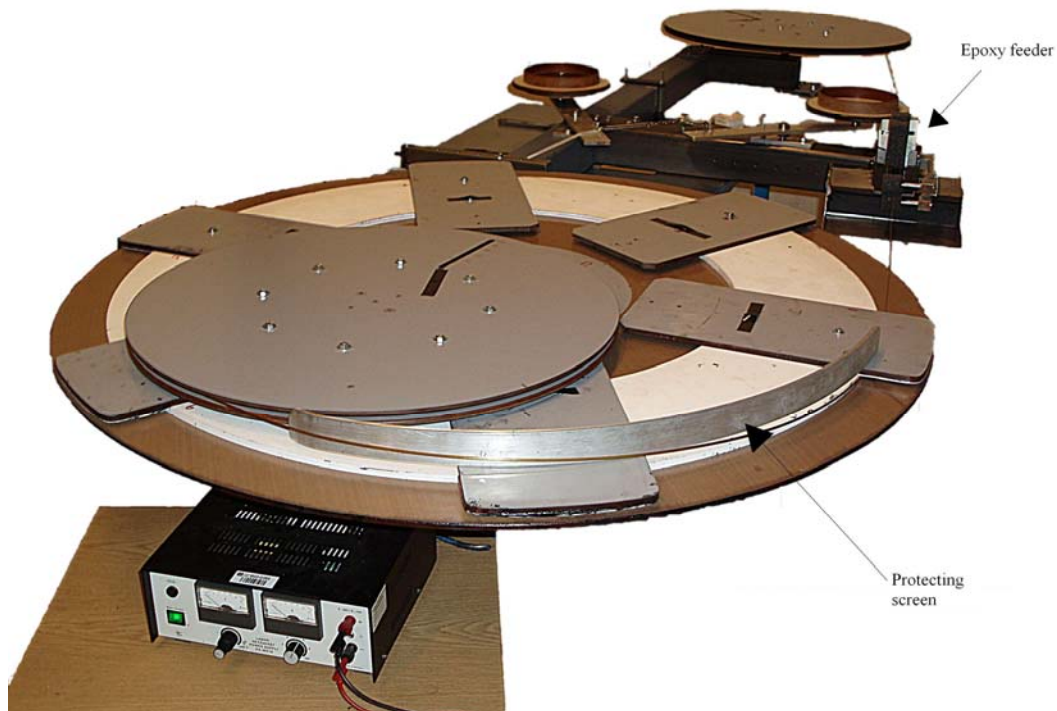
Figure 2-4: After removing 275 m the superconductor storage reel is moved to the edge of the winding table, the continuing part is placed under the first cover plate, the epoxy unit is put in position and the protective screen for the superconductor is assembled.
