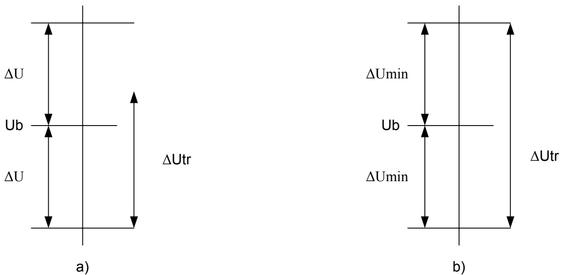
Figure 3.3: Sensitivity-settings for the transformer regulator, based on [10]
