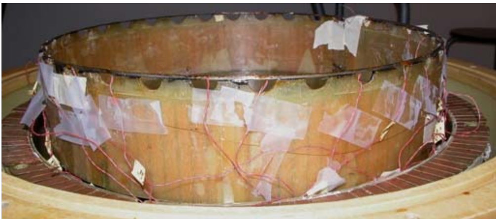
Figure 27 Picture of the holder and superconductors with copper wires and thermo elements glued onto them
