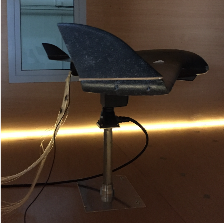
Figure 3.4: A sideways view of the tunnel setup with the Skywalker X8 mounted on the PTU-D48.
