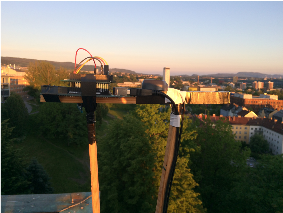
Figure 5.4: The sensor platform used to carry the Pozyx system next to the RTK-GPS. The antennas were 10,5 cm apart from each other.
