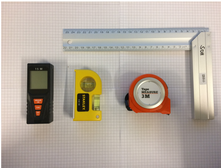
Figure 5.2: Tools used to measure the local coordinate system.
