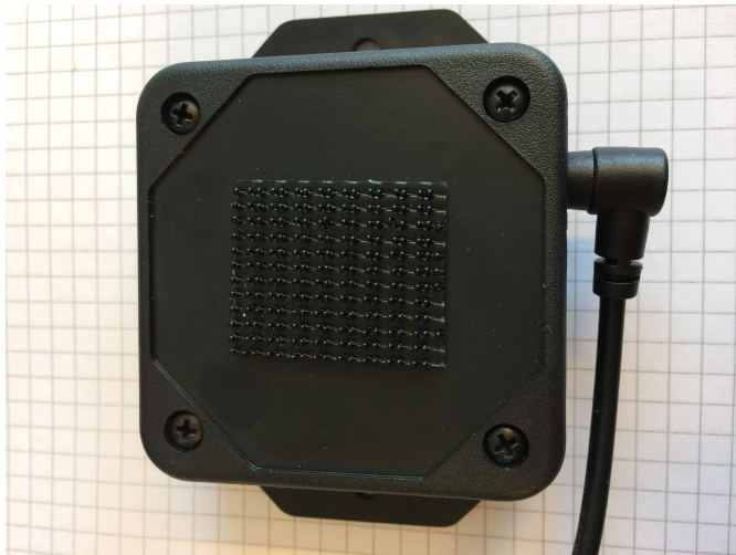
Figure 4.2: A Pozyx device configured to anchor mode.
