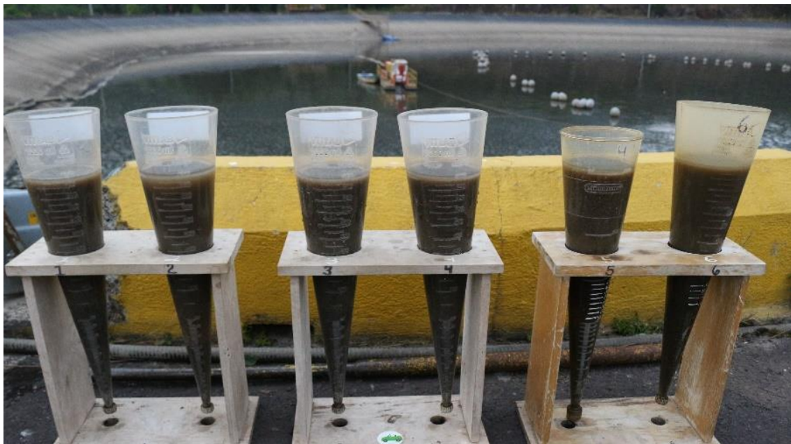
Figure 5.11 Measurement of sediment concentration at the discharge of the conventional dredge.
