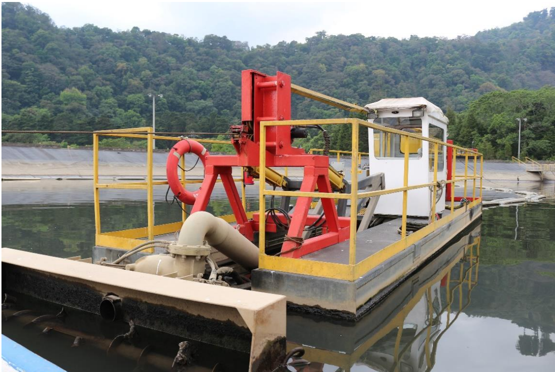
Figure 5.6 Conventional diesel dredge at El Canadá HPP.
