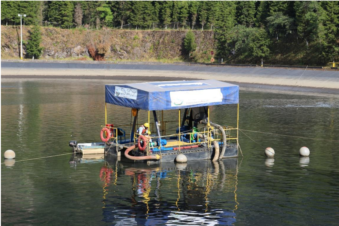
Figure 5.8 Hydrosuction dredge at El Canadá HPP.
