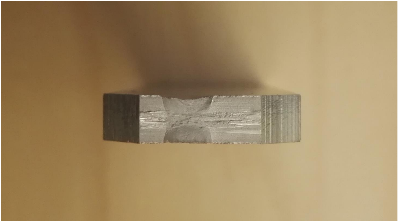
FIGURE 10 SPECIMEN 13, MAX LOAD 120 MPa, FATIGUE LIFE 116732 CYCLES, R=0.5
