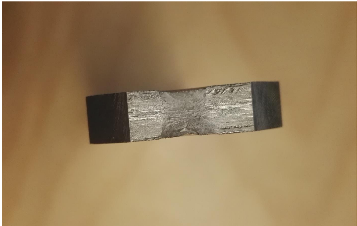
FIGURE 8 SPECIMEN 2, MAX LOAD 120 MPA, FATIGUE LIFE 16360 CYCLES, R=0
