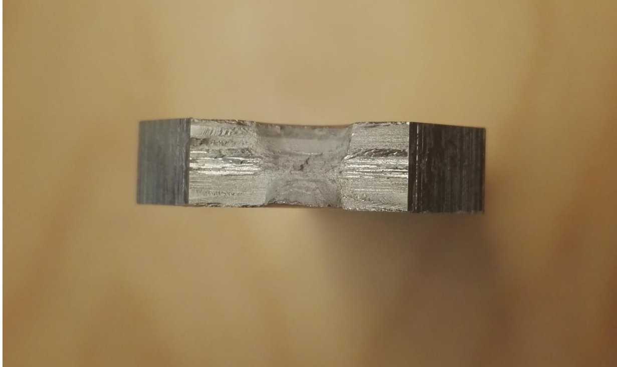
FIGURE 7 SPECIMEN 11, MAX LOAD 120 MPA, FATIGUE LIFE 16856 CYCLES, R=0
