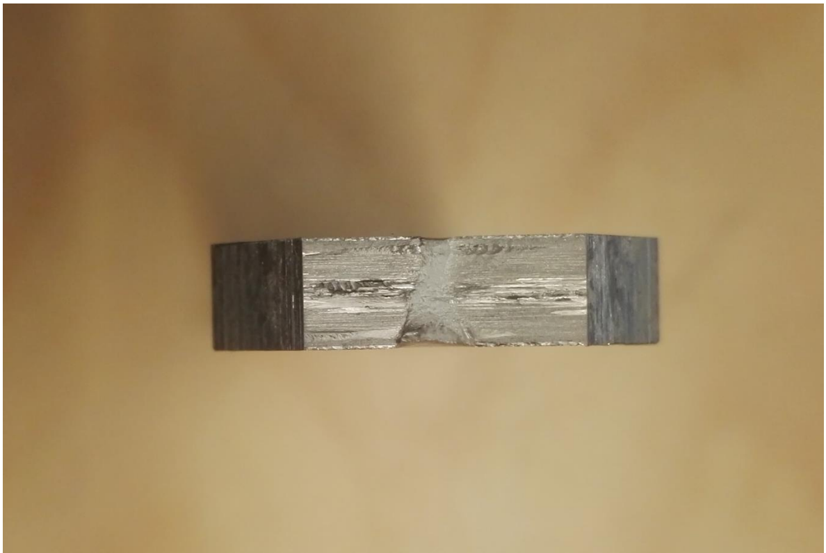
FIGURE 6 SPECIMEN 16, MAX LOAD 50 MPA, FATIGUE LIFE 532025 CYCLES, R=0
