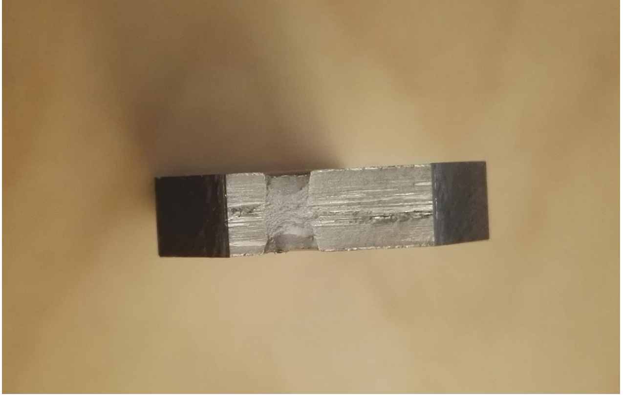
FIGURE 9 SPECIMEN 14, MAX LOAD 80 MPa, FATIGUE LIFE 653514 CYCLES, R=0.5
