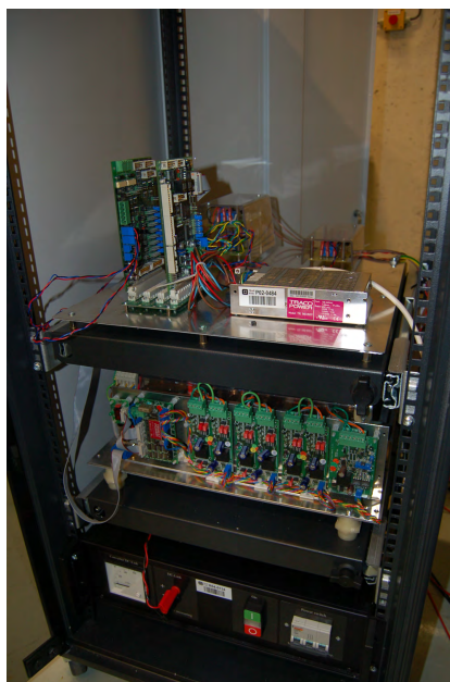
Figure 6.2.2: The back side of the converter, with driver circuits, DSP and measurement set up
