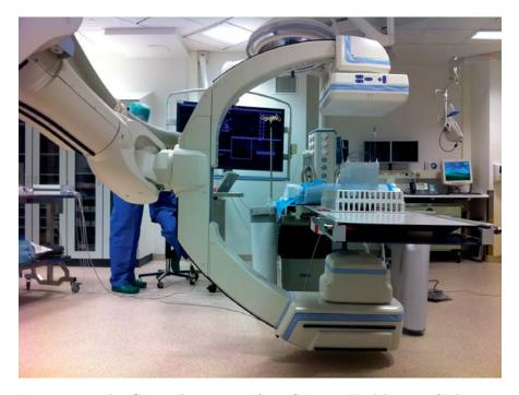
Figure 1.8: The C-arm Artis zeego from Siemens Healthineers (Erlangen, Germany) during imaging of an accuracy phantom. The C-arm is integrated with a floor-mounted robotic arm, which makes it very flexible, and can produce CT-like 3D volumes in addition to ordinary real-time fluoroscopic images.
