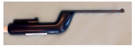
Figure 5.3: Prototype ultrasound probe for pituitary and spine surgery with a curved array, which allows for imaging to the side and forward at the same time.
