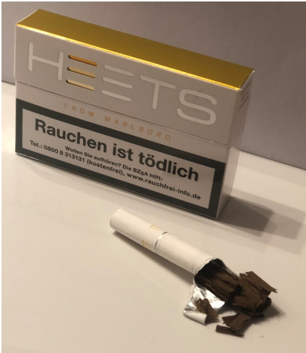
Figure 15 Heets: What the specialized tobacco looks like on the inside, along with the aluminum that prevents combustion
