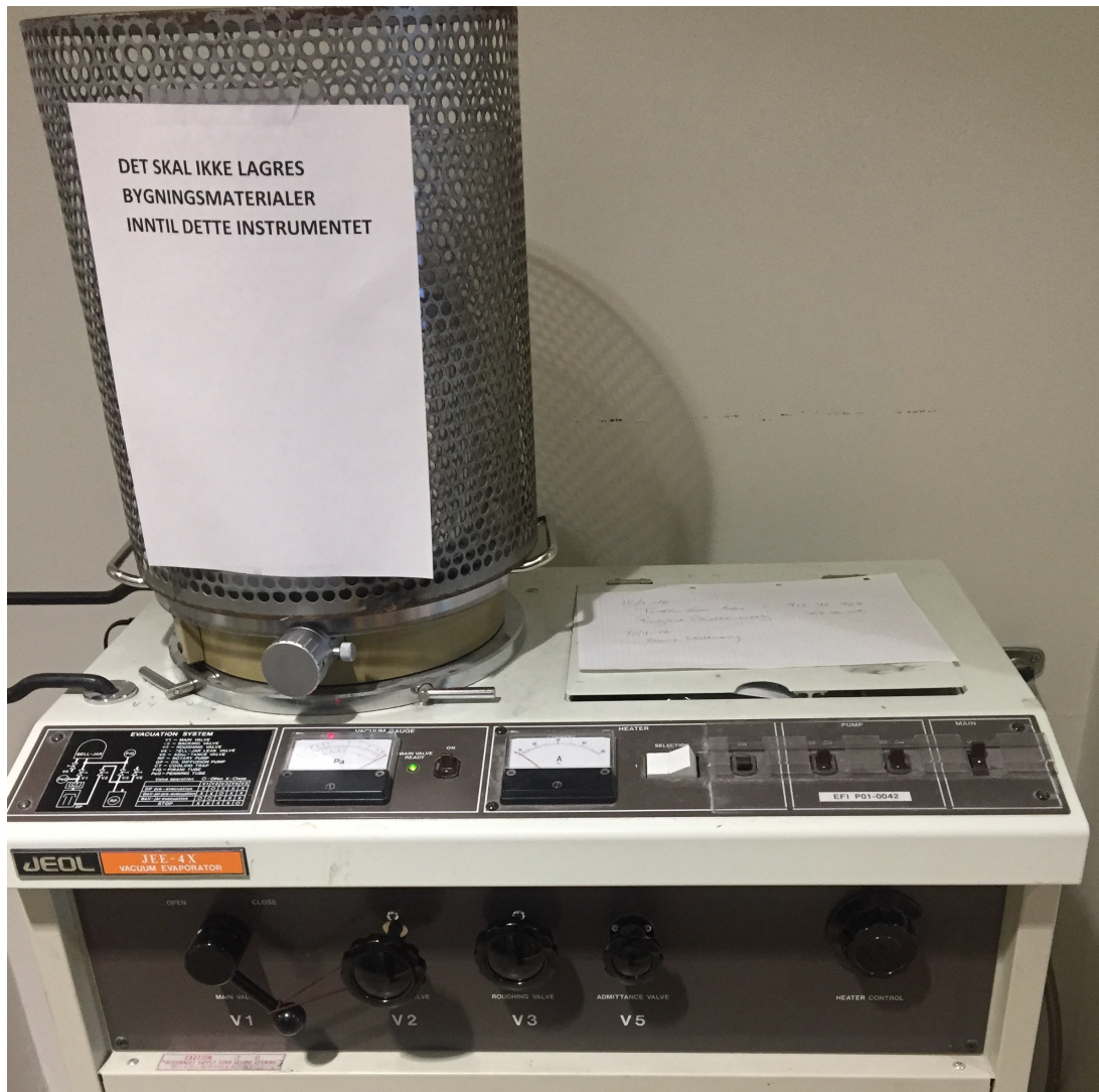
Figure B.1: The vacuum evaporator while in operation. The bell jar is protected by a plastic and metal shield.
