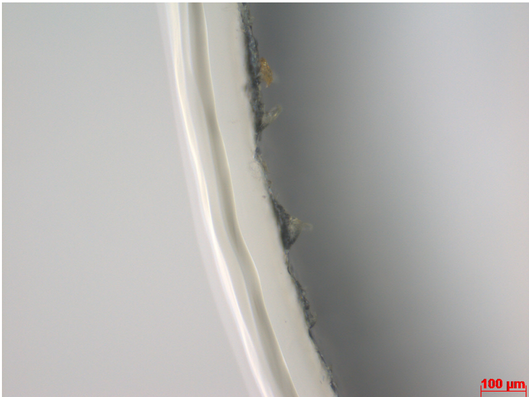
Figure L.11: The figure shows the edge of the 20 mm void in polycarbonate.
