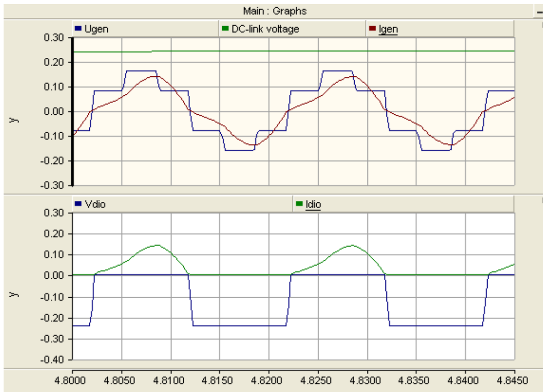
Figure 64: Simulated generator phase voltage [kV], generator current [kA], diode current [kA] and diode voltage [kV] for 50Hz generator frequency and without reactive compensation
