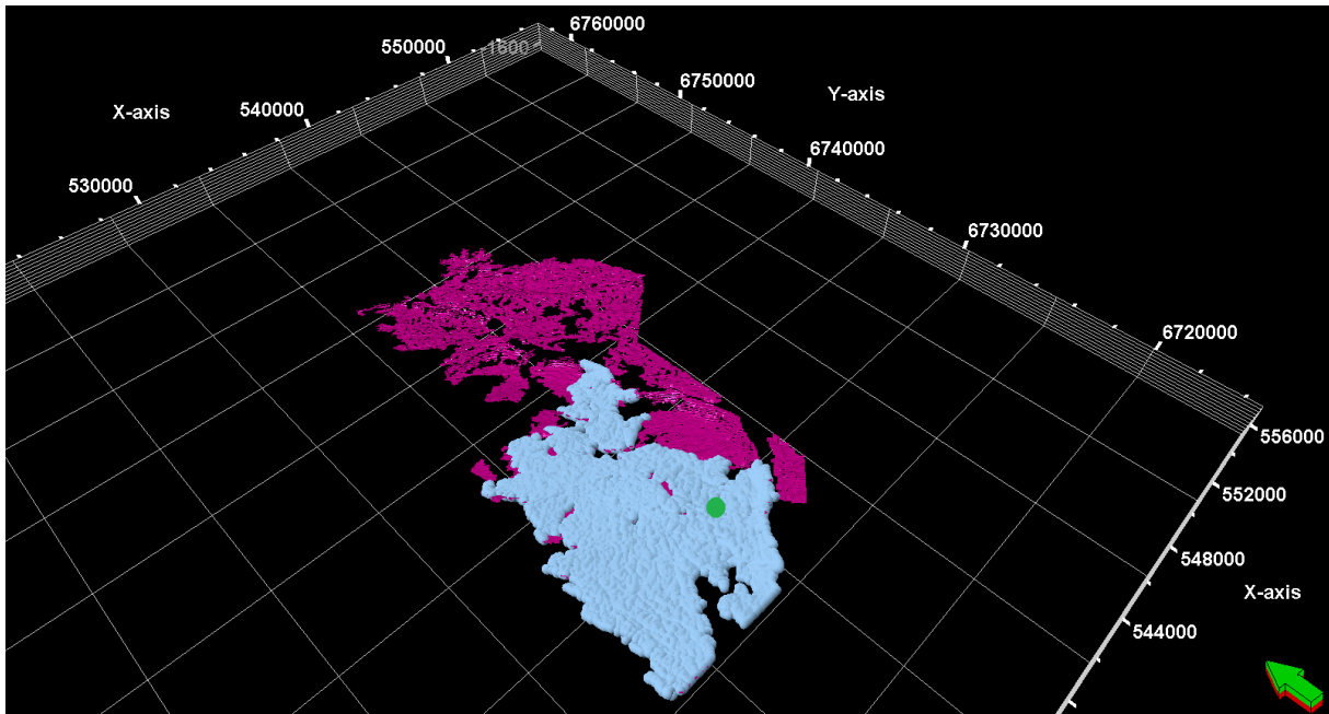
Figure 55: A comparison between the IntelliTracker and the Basic 3x3 Horizon Autotracker. The blue point set surface represents the IntelliTracker, while the pink smooth
