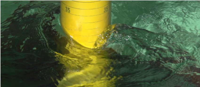
Figure 1.3: Example of water run-up behind the cylinder as a wave crest passes (Kristiansen and Faltinsen (2017)).
