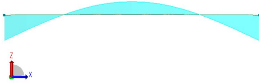
(a) Net moment distribution of bending moment about y-axis due to forces applied in z-direction.
