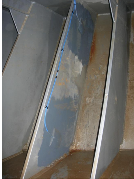
Figure 18: Sensors mounted on hull structure (Leira & Børsheim, 2008).
