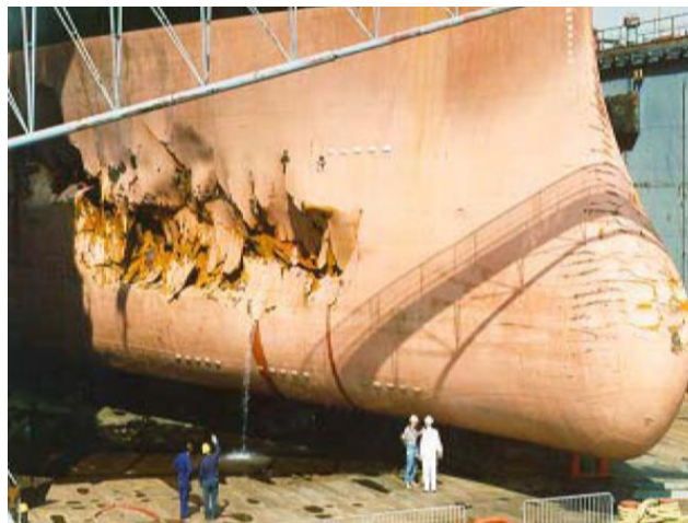
Figure 9: Damage from collision with ice features (Riska, 2017d).
