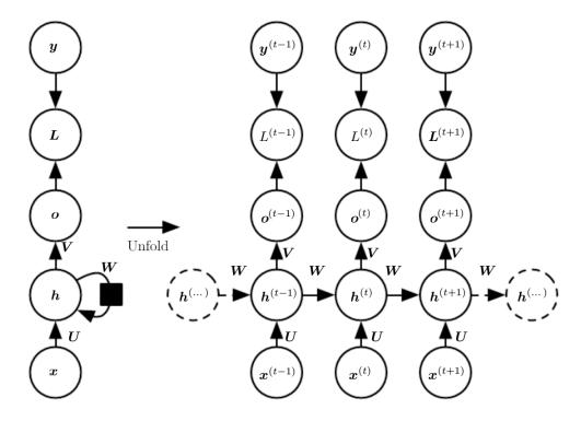
Figure 3.6: Circuit Diagram and Unfolded Computational Graph of General Recurrent Network (Goodfellow et al. (2016) Figure 10.3 Section 10.2)
