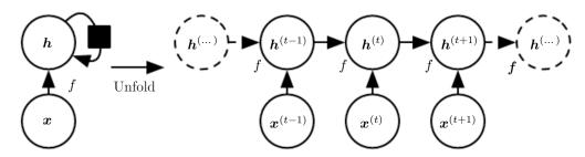
Figure 3.5: Unfolded Computational Graph and Circuit Diagram Representation (Goodfellow et al. (2016) Figure 10.2 Section 10.1)
