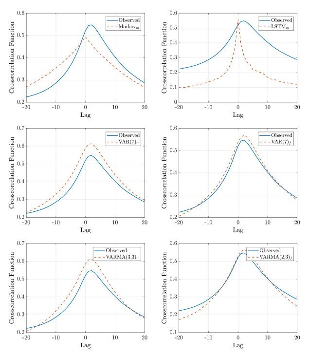
Figure B.5: Comparison Plot of Crosscorrelation Function for North Sea Series
