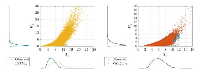
Figure 6.3: Validation Scatter Plot of  $H_s$  and  $T_p$  for Mediterranean Sea Series
