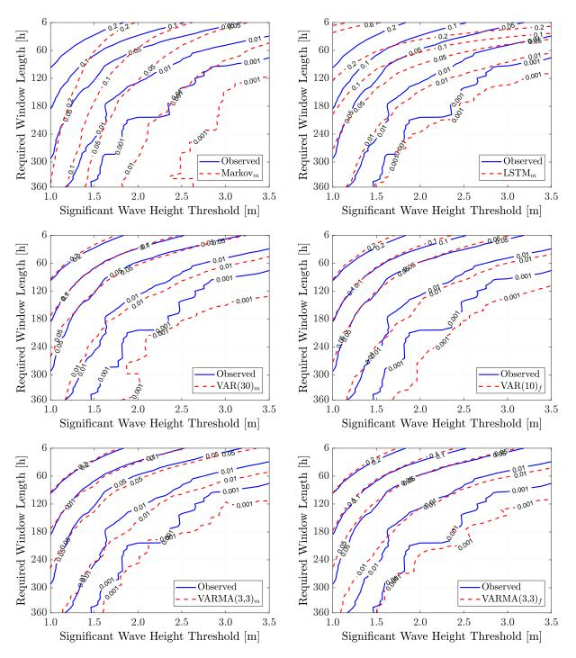
Figure B.13: Comparison Plot of Normalized Persistence Above Threshold Contours for Mediterranean Sea Series
