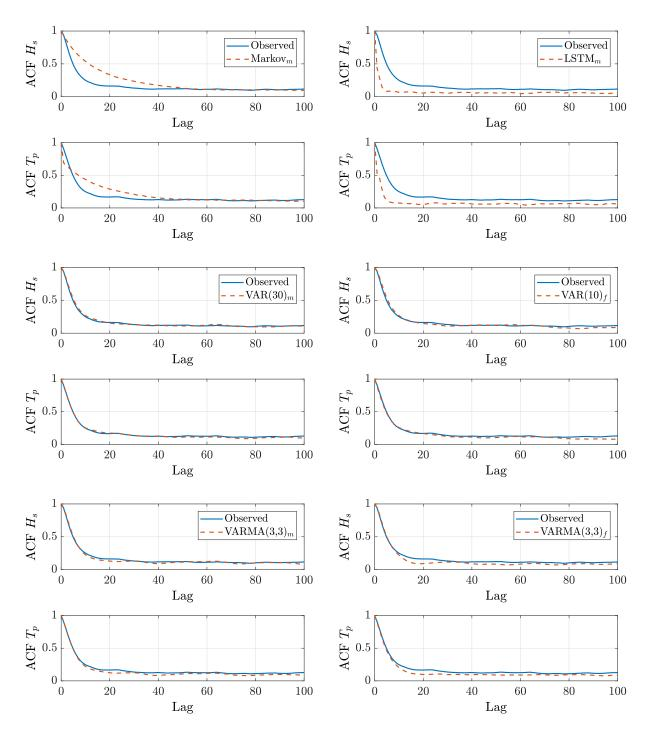
Figure B.11: Comparison Plot of Autocorrelation Function for Mediterranean Sea Series
