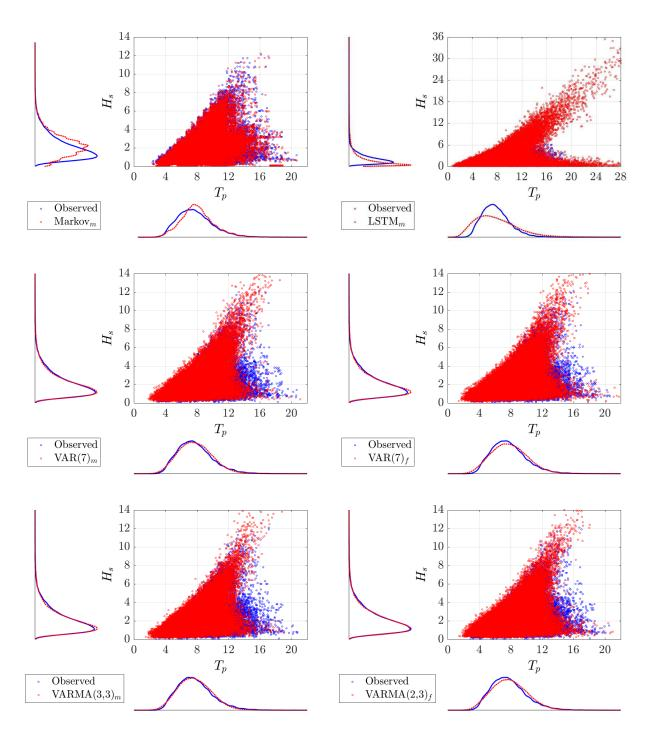
Figure B.3: Comparison Plot of Joint and Marginal Distribution for North Sea Series
