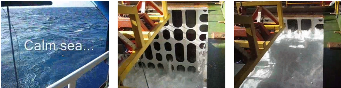
Figure 1.2: Snapshots from video showing calm sea conditions, while moonpool operations were not possible due to resonant flow (Kristiansen et al., 2013)
