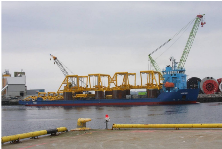
Figure 2.1: SPS structure is loaded onto the operation vessel (ref: [3])
