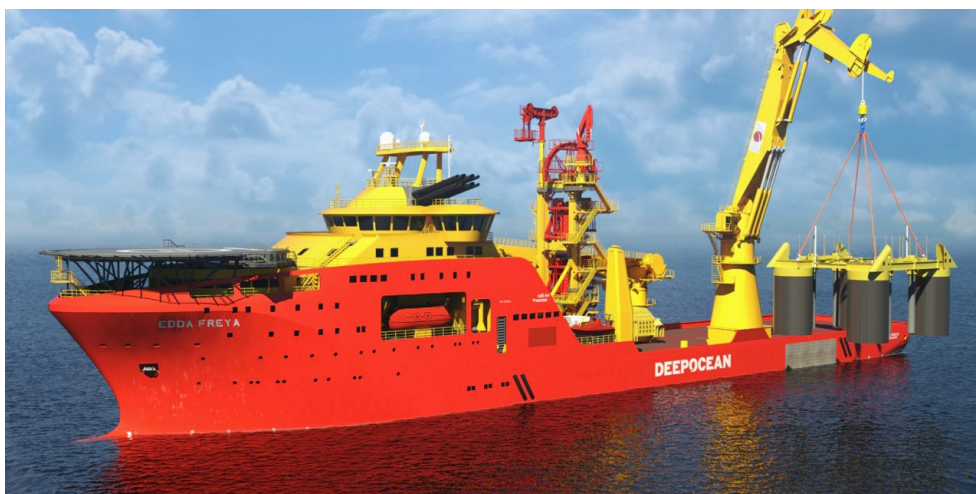
Figure 2.2: Lifting of the SPS over the side of the ship and through splash zone (ref: [4])
