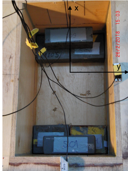
Figure 3.2: Weight distribution of the ballast weights in the model. The weights are placed symmetrically around both the x-axis and the y-axis.
