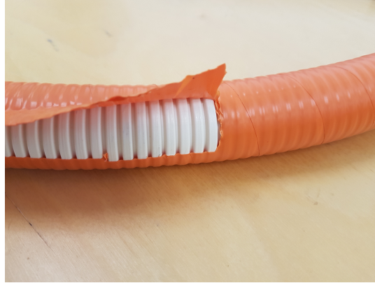
Figure 3.2: Corrugated tube enclosed by water repellant tape.
