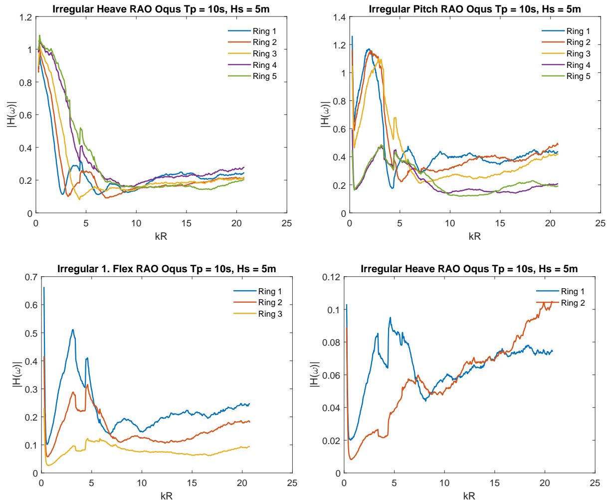
Figure 5.9: Experimental RAO results in heave, pitch, first and second flexible mode in using motion capture markers on ring 1, 2, 3, 4 and 5, in irregular waves with T_p = 10s and H_s = 5m .
