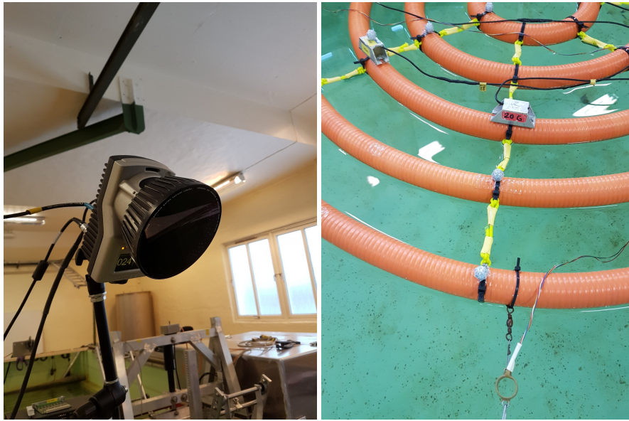
Figure 3.5: The Oqus Camera, used for measuring the x,y,z -position of the 24 motion capture markers at 200 Hz. Equipment and instruments used to measure movement, force and acceleration of the model.
