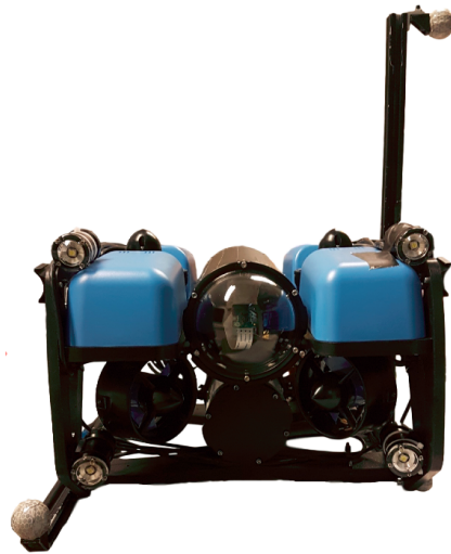
Figure 5.4: BlueROV with markers for Qualisys camera system
