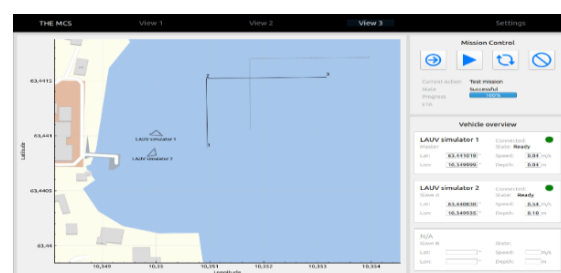
Figure 4: View 3 of the MCS. The view for starting mission execution and monitoring mission execution.
