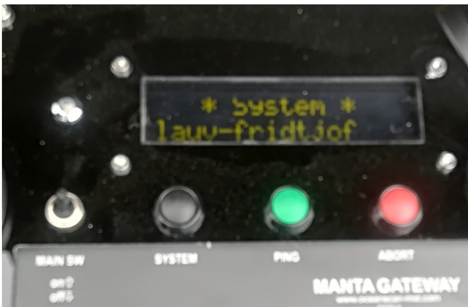
Figure 3.6: The Manta up close depicting the information screen and switched and buttons available.
