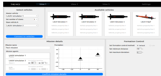
Figure 2: View 1 of the MCS. For defining the vehicle team, formation, and constraints.
