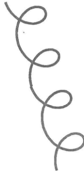
Figure 4.4: Trajectory of a particle with a constant velocity and rotating due to impact from the Coriolis force, only. Illustration from Mellor (1996).
