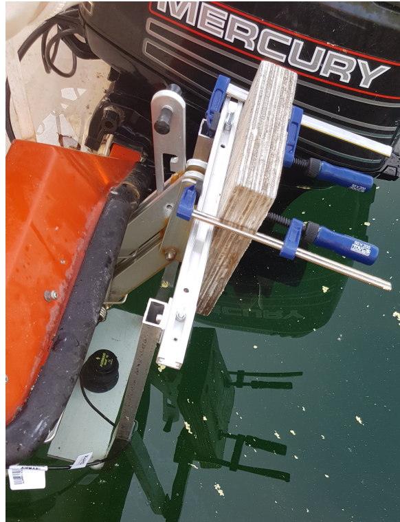
Figure 4.42: Mounting echo sounder to boat
