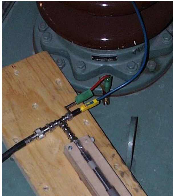
Figure C.2: Setup using active probe to measure applied voltage
