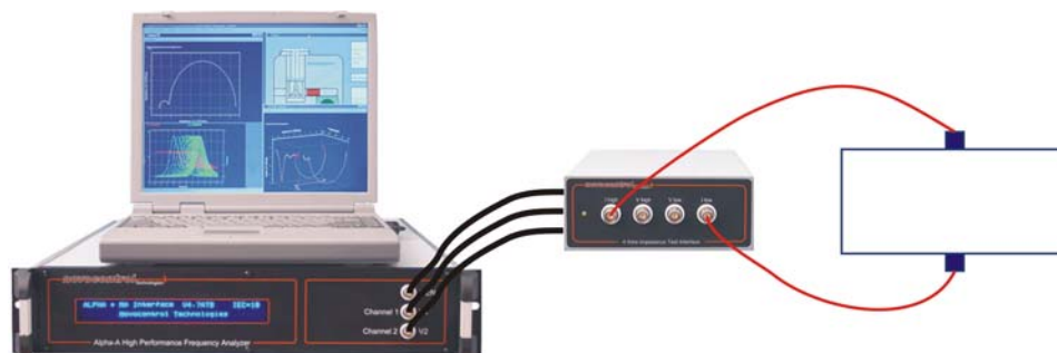
Figure 6.2: Novocontrol Alpha analyser, ZG4 test interface, laptop and test cell
