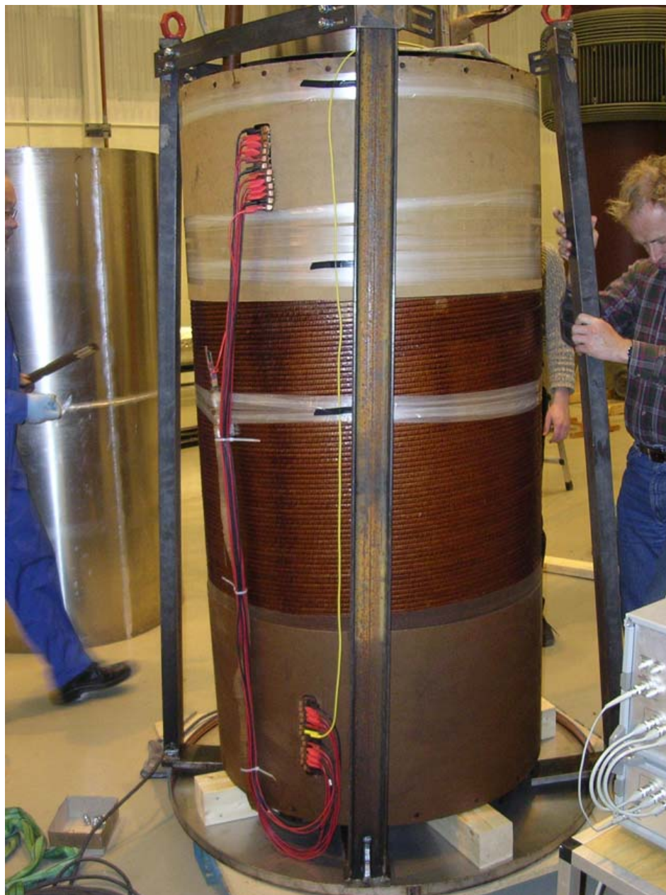
Figure K.2: Axial displacement on T3Buran winding
