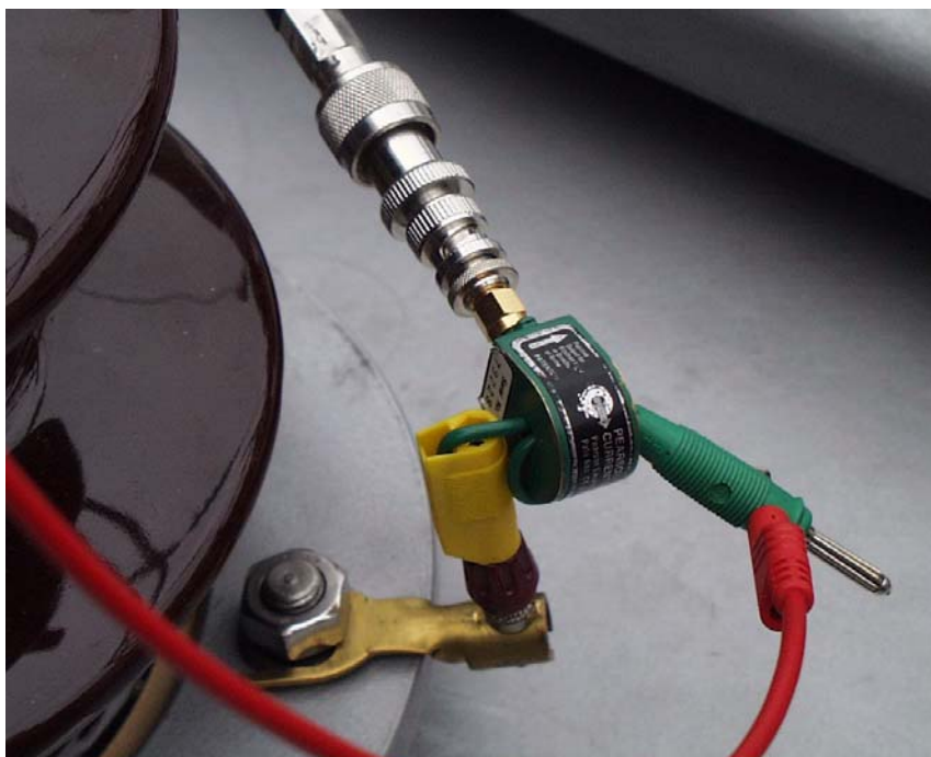
Figure C.3: Current measurement using a Pearson Current monitor
