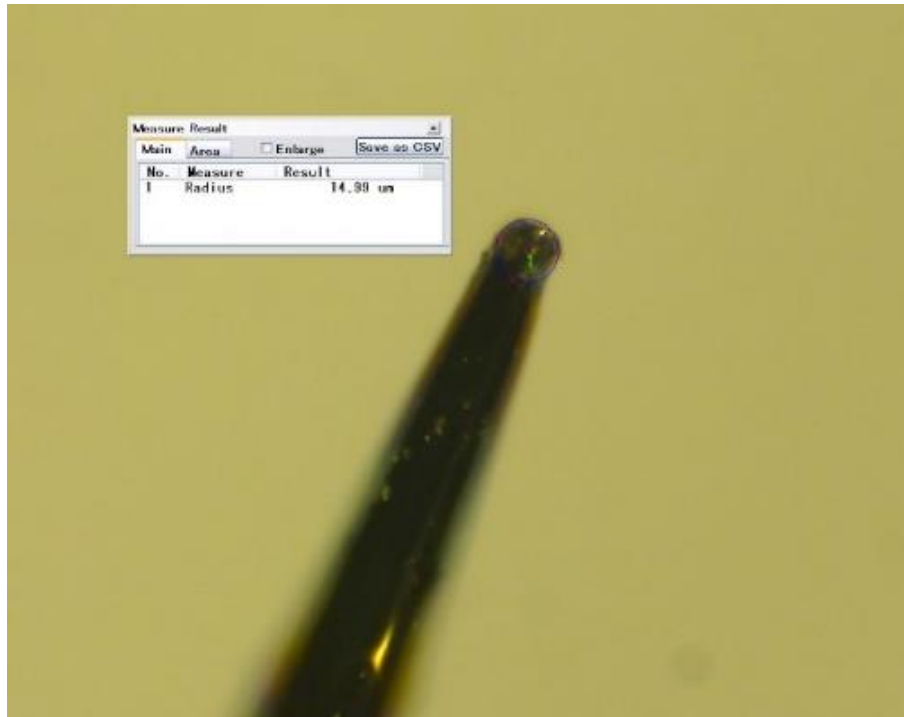
Figure 31. Microscope photo of the tip ( 15\mu\text{m} radii) before the experiment shown in figure 20.
