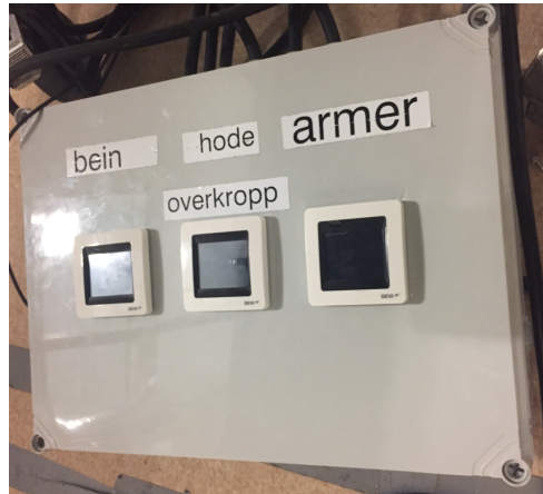
Figure 51: Control panel for the surface temperature of the manikin
