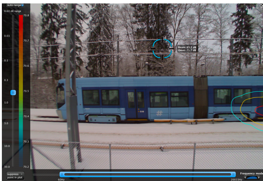
Figure 4.6: Acoustic camera measurement of third vehicle on SL-95 tram at height B.
