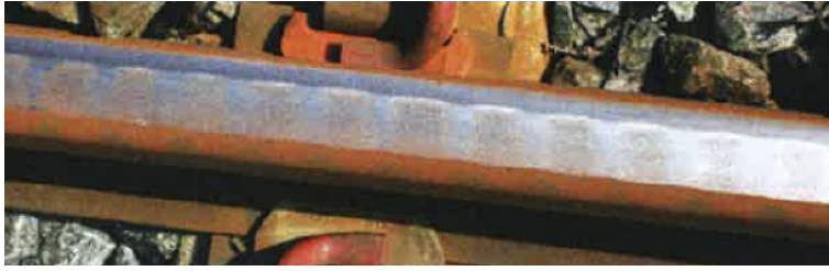
Figure 2.5: Rail corrugation on rail on one part of the metro tracks in Oslo [12]
