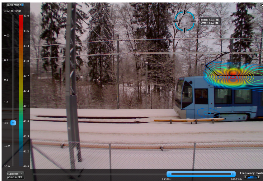
Figure 4.7: Acoustic camera measurement of first vehicle on SL-95 tram at height B with frequency spectrum from 2kHz to 20kHz
