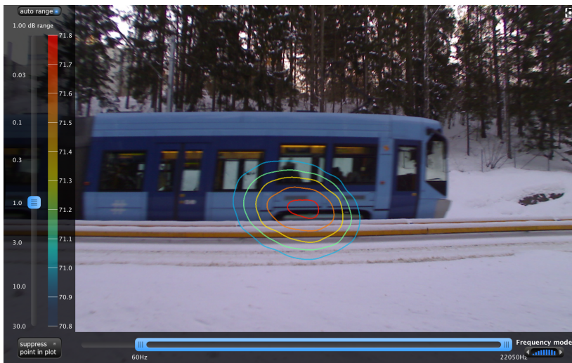
Figure 4.3: Acoustic camera measurement of third vehicle on SL-95 tram at height A.
