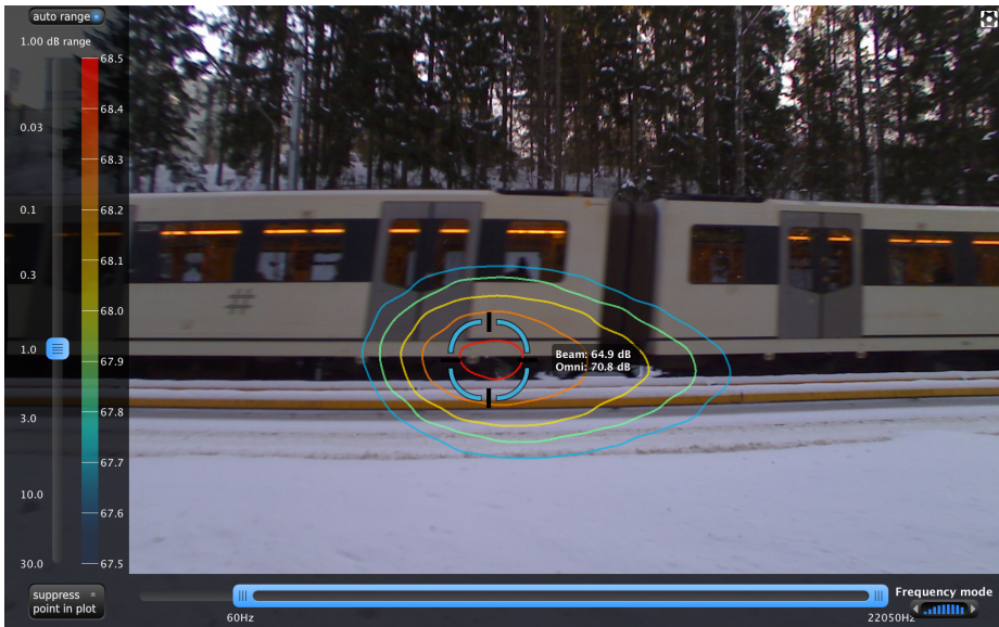
Figure 4.10: Acoustic camera measurement of second and third vehicle on MX3000 train.
