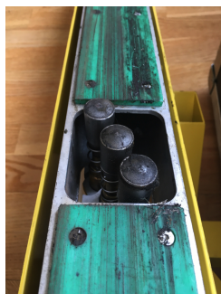
Figure 3.9: Three displacement sensors on the rail side of the rail surface analyser.
