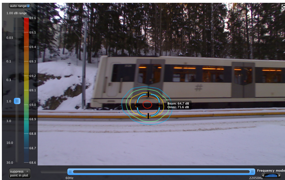
Figure 4.8: Acoustic camera measurement of first vehicle on MX3000 train.
