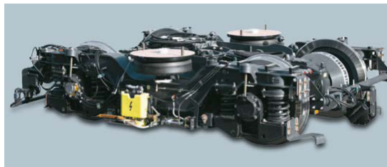
Figure 3.3: MX3000 boogie with visible brake disks and traction motor.
