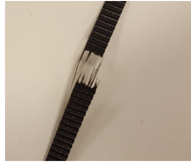
Figure 7.4: 9mm HTDM5 belt snapped
