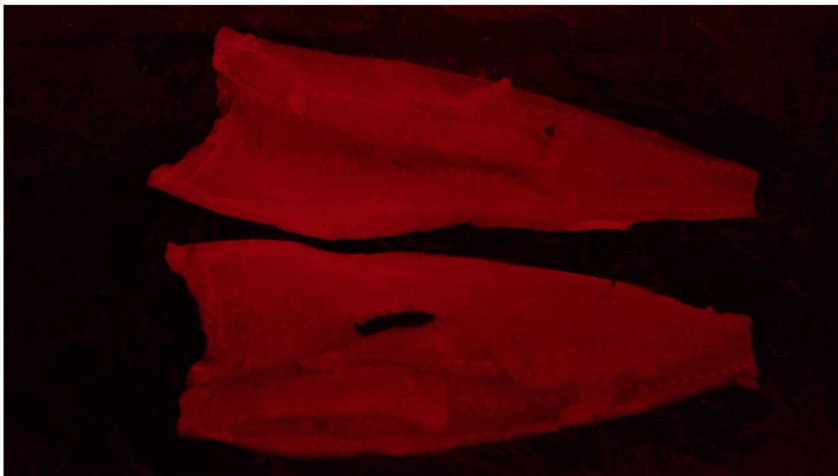
Figure 4.26: Red illuminated fillets (640nm).
