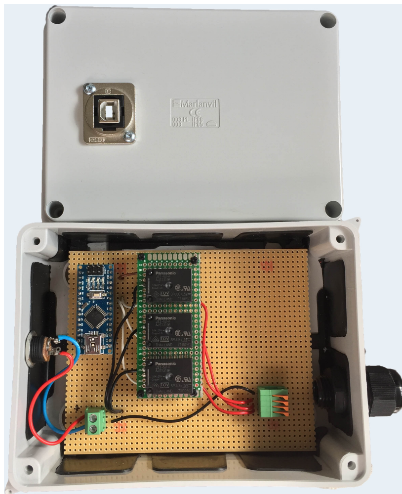
Figure 4.12: Light controller box
