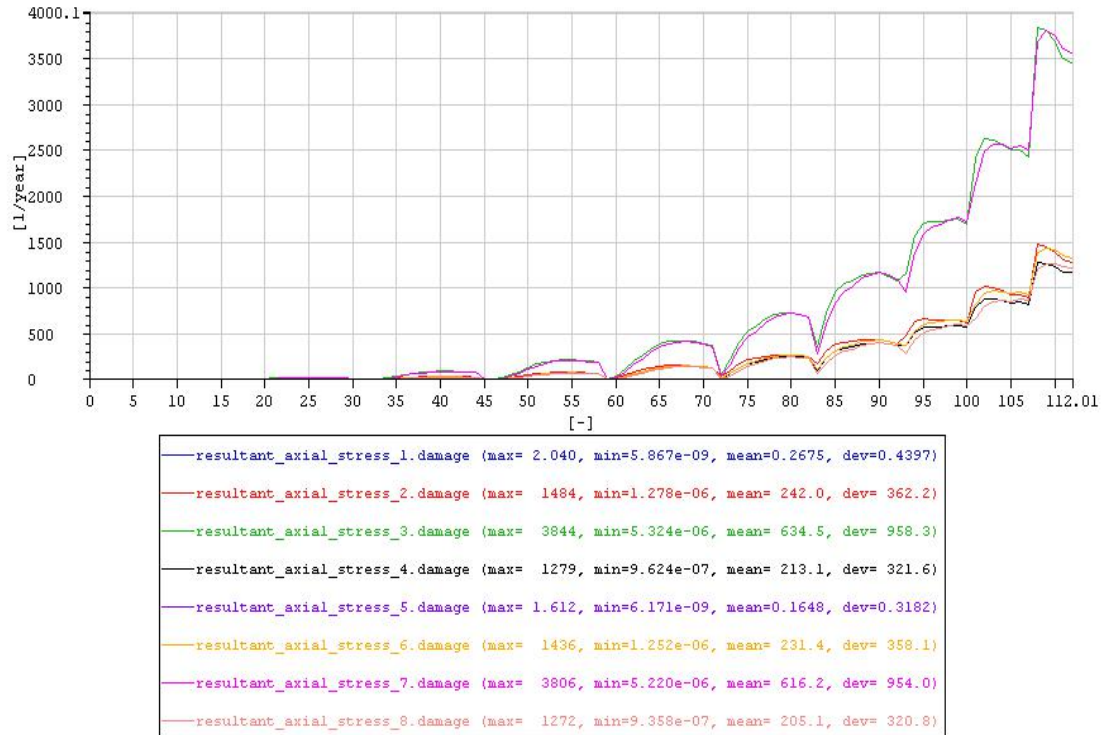
Figure 7-9. The fatigue life of riser with fixed topside connection by resultant stress.
