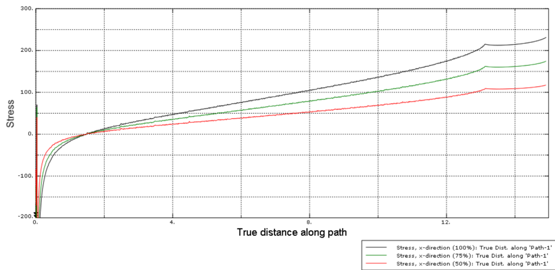
Figure 5.14: Stress in the x-direction along the contact surface 0.3 friction
